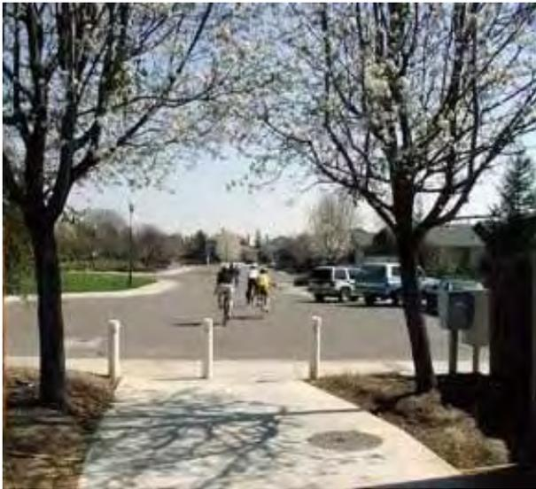
Multi-use trail access point can be limited with bollards. Bollards prevent motorized vehicles from entering the path while allowing bike/ped access.
